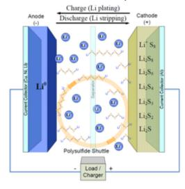
The "ions" can be provided by a number of materials including Sulphur and Oxygen. A Li-S battery has a lithium anode and carbon-sulphur cathode. Again the lithium ions transfer to the cathode during discharge. The Li-S battery can be punctured (with a nail!) in safety – it does not explode like a Li-Ion battery. Li-S batteries have low weight and can provide over twice the storage capacity of Li-Ion (a sulphur atom can contribute 16 electrons). They are still under development.
